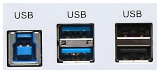
Fig. 3.32 USB Connector (type B configuration on the left and type A configuration on the right)
