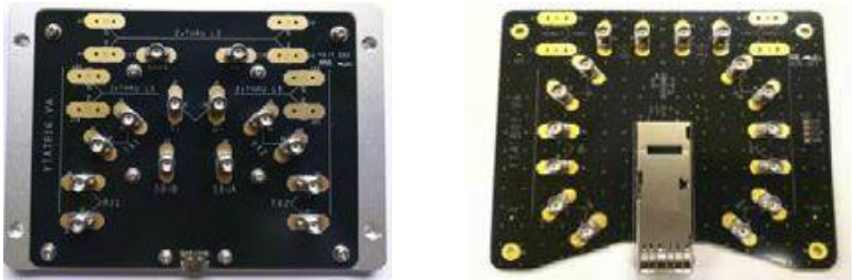
Figure 4.3 Test fixture for connectors (Type-C on the left, QSFP+ on the right)
